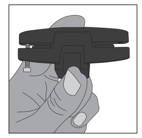
**1.** Take one of the screws out of the click system. Loosen the other screw to the end of the nut.
